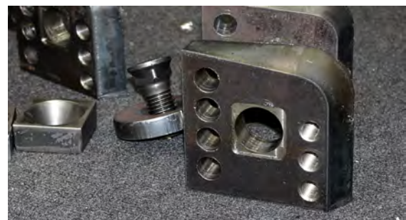
Fig. 9 - Cut Sample with Flood Coolant. Oil covered surface can be avoided with MQL
