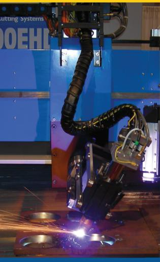
The PCS Plasma Bevel Head is designed and manufactured by Profile Cutting Systems (PCS) This PATENTED and revolutionary design has taken the metalworking industry by storm! Unlike other cumbersome, rotary type bevel heads, the PCS Bevel Head is compact, lightweight and FAST. It sets a new standard in Plasma Bevelling Technology.
