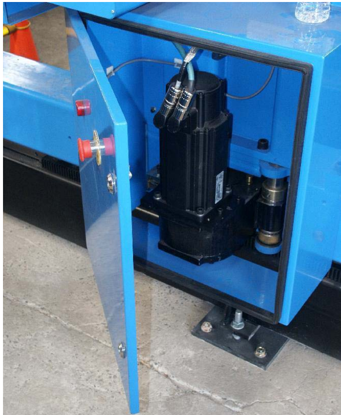
PCS Heavy Duty Longitudinal Motor Gearbox assembly
